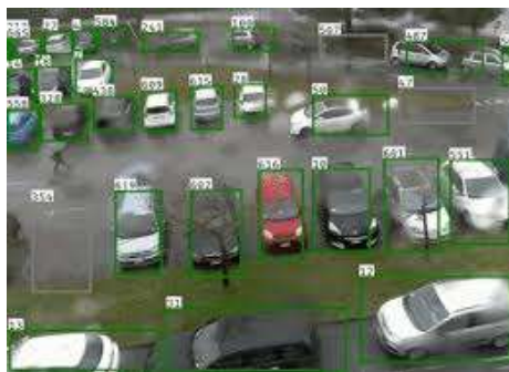
Figure (10) Detection of stationary vehicles
