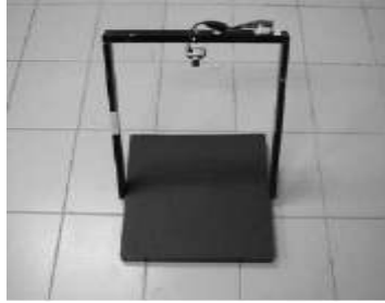
Fig 4. The stand of fruit image acquisition system Aibinu et al. (2011).
